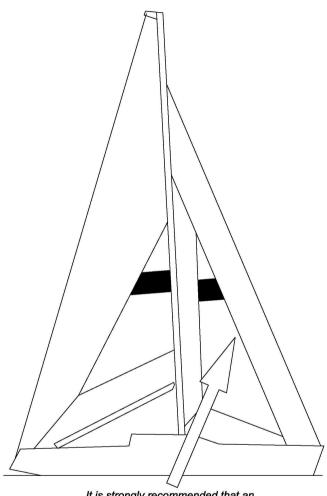
It is strongly recommended that an inner forestay is provided either permanently installed or readily set up, on which to set the storm jib
